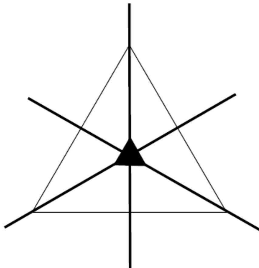
The equilateral triangle allows six symmetry operations: rotations by 120 and 240 around its centre, reflections through the three thick lines intersecting the centre, and the identity operation.
