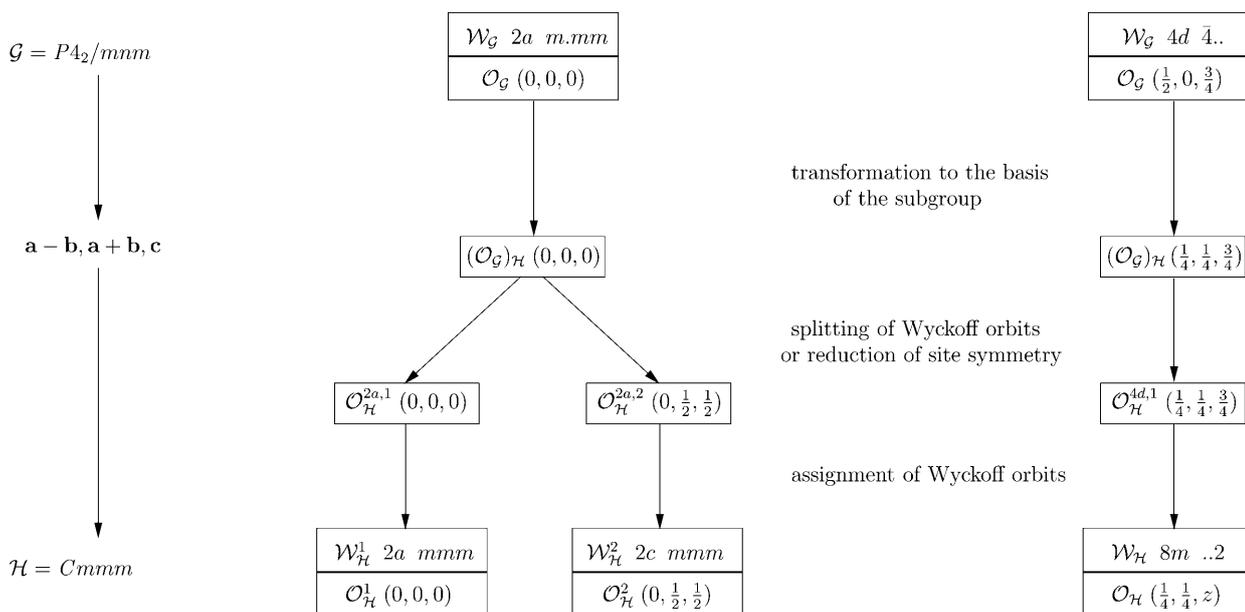
**Fig. 7.** Splitting of the Wyckoff positions  $2a m.mm$   $(0, 0, 0)$  and  $4d \bar{4}..$   $(\frac{1}{2}, 0, \frac{3}{4})$  of  $P4_2/mmm$  with respect to its subgroup  $Cmmm$  of index 2.  $(\mathcal{O}_{\mathcal{G}})_{\mathcal{H}}$  are the orbits of  $P4_2/mmm$  in the basis of  $Cmmm$ .
