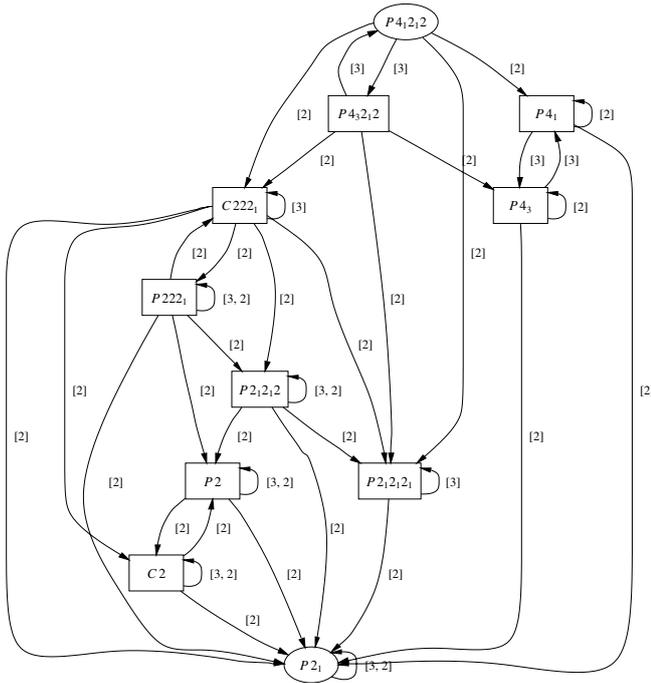
**Fig. 3.** General contracted graph for  $P4_12_12 > P2_1$ . The nodes of the graph correspond to the types of space groups that can appear as intermediate subgroups in the chains of the group-subgroup pair  $P4_12_12 > P2_1$ . Each edge of the graph corresponds to a group-maximal subgroup pair of the indicated index  $[i]$ . The loops correspond to isomorphic subgroups.
