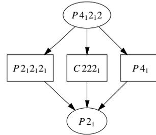
**Fig. 4.** Contracted graph for the pair of space groups  $P4_12_12 > P2_1$ , index 4. The nodes correspond to space-group types. The directed edges represent the possible group-maximal subgroup pairs.
