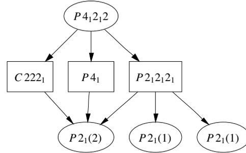
**Fig. 5.** Complete graph for  $P4_12_12 > P2_1$ , index 4. The nodes represent space groups and not space-groups types. The three subgroups of the type  $P2_1$  are distributed into two classes of conjugate subgroups which are indicated in the parentheses after the space-group symbol. The two subgroups  $P2_1(1)$  belonging to the same conjugacy class have identical single graphs, which considerably differ from the graph of  $P2_1(2)$ .
